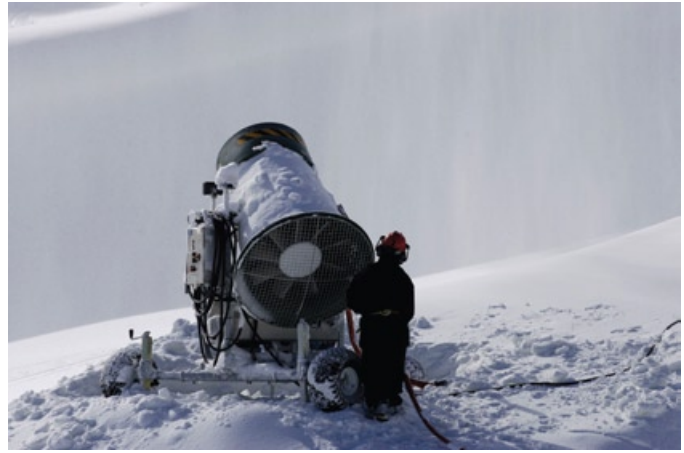
One of the snowmaking “guns” powered by the micro-grid ensures a solid snow base throughout the ski season.
