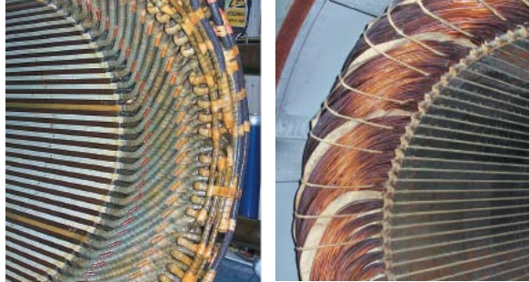
Figure 2 - Stator assembly of bar-wound machine (left) and wire-wound machine (right). Note the difference in slot size and bracing wiring on wire-wound machine.
